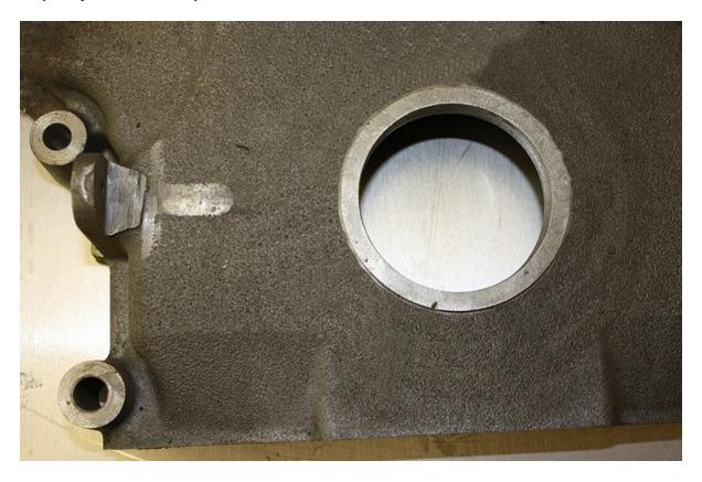
Measure over 4.140" from the center of the crankshaft and make a mark on the crank sensor mounting boss. This mark will indicate how much of the boss must be removed for proper clearance. The boss must be ground down to within .070" of the surface of the timing cover for proper clearance on the rear of the damper. We also suggest checking the height of the
